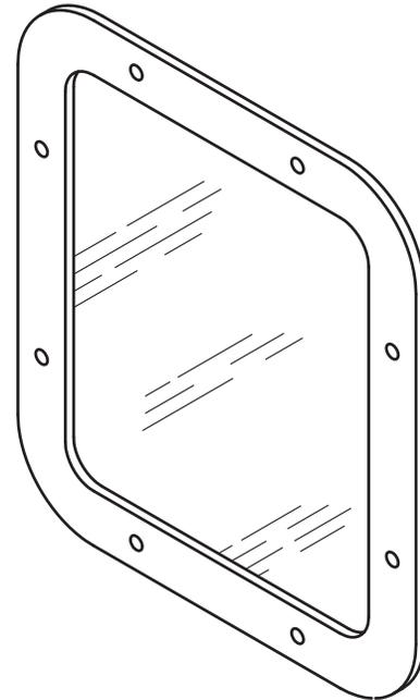
**MR** \_\_\_ mirror with integral frame shall be die formed 16 GA, Type 304 series stainless steel, polished to a #8 non-directional mirror finish. Anchoring shall be by standard 8-point mounting. Vandal-resistant security screws provided with the mirror. Wall anchors provided by others.
