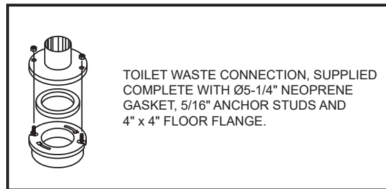
(TW4) FLOOR OUTLET WASTE CONNECTION
