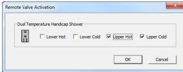
Figure 35 - Remote Valve Activation for Dual-Temp Handicapped Shower
