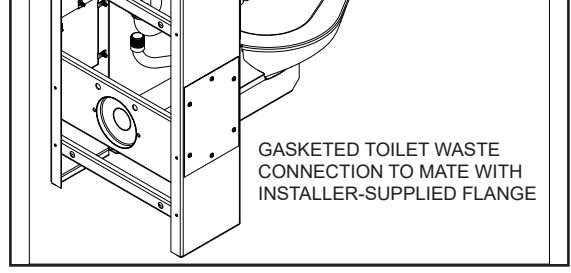
(GWC)- GASKETED WASTE CONNECTION (WALL OUTLET SHOWN)
