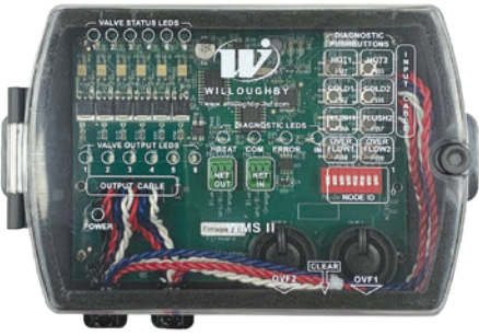
Willoughby Cell Valve Controller (CVC) in water-resistant enclosure
